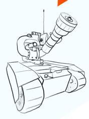
Heavy-duty firefighting robot TrackReitar HD is designed for firefighting in very complex environments such as forest fires, industrial fires, etc.
